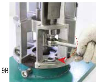
**20** Use TORQUE WRENCH and FIXTURE FOR STRAP to tight at correct torque (clockwise)
