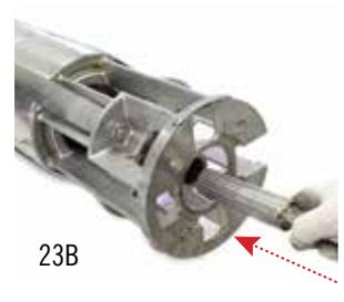
**24** Use **Depth Caliper** to check shaft clearance
