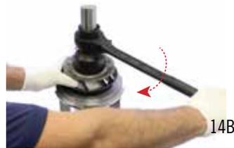
Use TORQUE TESTING NUT and WRENCH to tight at correct torque (clockwise) (Step 9)
