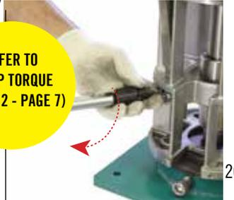
**21** Remove **SCREWS** to loosen **JIG**
