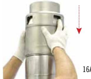
**17** Make sure bolts on discharge are aligned with bolts in INTERCONNECTOR
